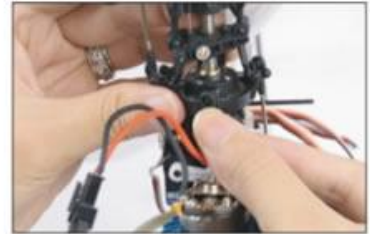
18. 将前后升降伺服器拉杆连上 Link up all the push-rods on the front & rear servos.
