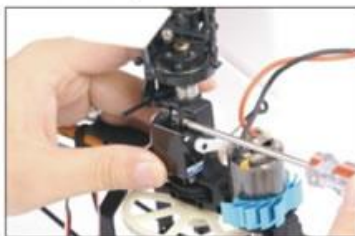
2. 将前后升降伺服器固定 Fix the front and rear ELE servoes.
