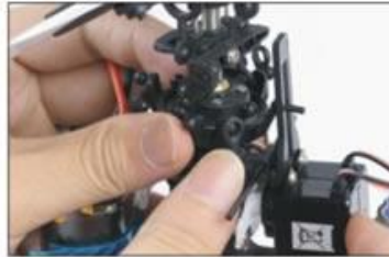
17. 将左右伺服器拉杆连上 Link up all the push-rods on the left right servoes.
