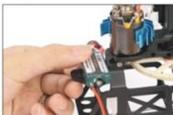
5. 将调速器用双面胶粘好 Stick up the ESC with double paste.
