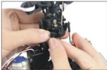
19. 将螺距伺服器拉杆连上 Link up the push-rods on the pitch servo.
