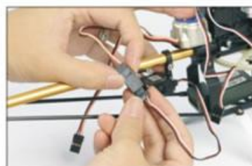
9. 将陀螺仪和方向伺服器连接 Connect the gyro and motor.
