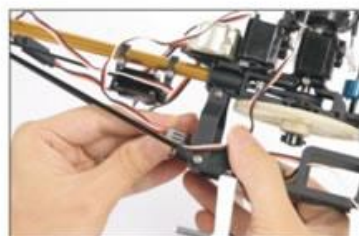
15. 将螺距伺服器连接在第六通道 Connect the pitch servo with CH6.
